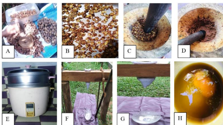
Fig. 4: Steps followed in C. inophyllum seed oil extraction on a small scale, starting from kernel to separation of oil. A: Dried nuts were deshelled to expose the kernel. B: Sliced kernels were dried. C: Dried kernels were ground. D:
